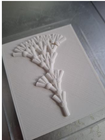
Figure 9 - 3D printed L-system
