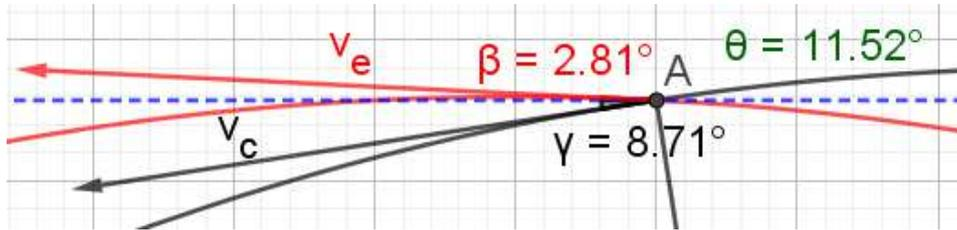
$$\Delta V^2 = \|\vec{v}_e - \vec{v}_c\|^2 = \|\vec{v}_e\|^2 + \|\vec{v}_c\|^2 - 2\|\vec{v}_e\| \times \|\vec{v}_c\| \times \cos(\theta)$$
