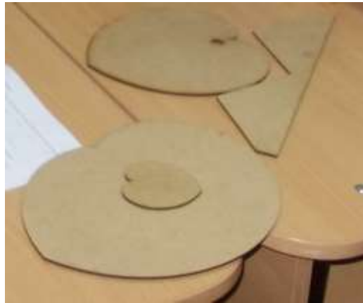
Image 3. Plywood model of a shaped serrated road and bicycle wheel
